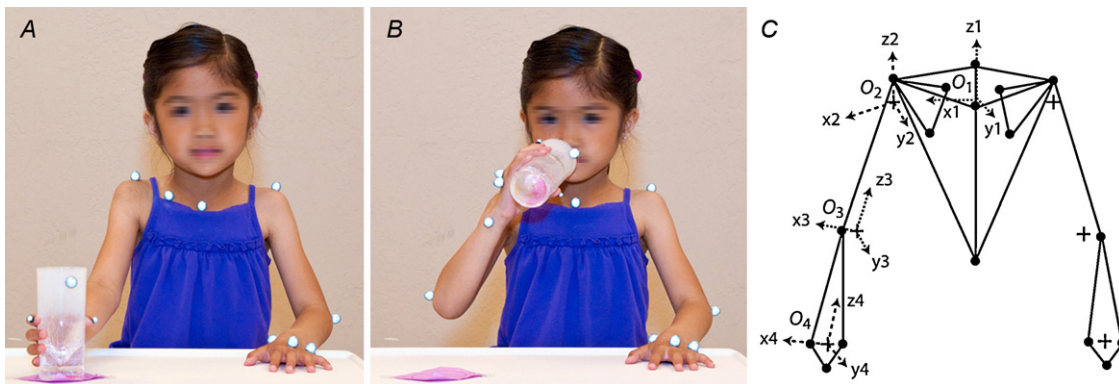
Fig. 1. Typically developing participant demonstrating the testing set-up and placement of the retro-reflective markers while (A) reaching forward to grasp the cup and (B) transporting the cup to the mouth. The segmental coordinate systems for the trunk and upper limb (C) using estimated joint centers as local origins: trunk ( O_1 ), glenohumeral joint ( O_2 ), elbow joint ( O_3 ), and wrist joint ( O_4 ).
